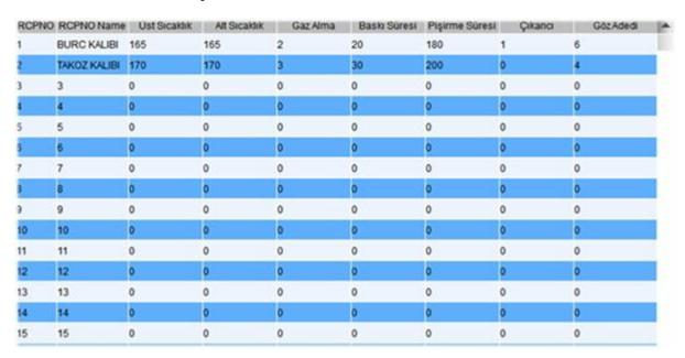
You can save 1000 molds with their names and all their parameters on our presses. When changing molds, you can adjust all parameters simply by selecting the mold.
