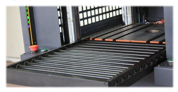
The sliding front stand on our ECO series presses makes it much easier to place and remove molds. It can also be easily removed if desired.
