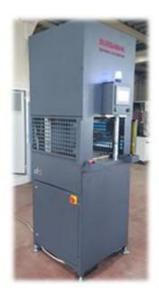
All hydraulic and electrical components of our presses are self-contained, allowing them to take up minimal space in your production area.
