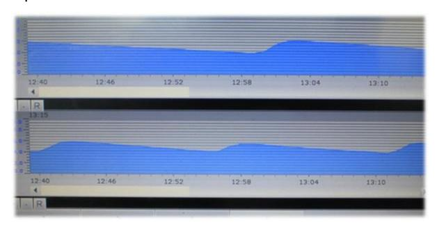
Our presses record the upper and lower table temperatures for the past hour and present them in a graphical format. You can monitor temperature values minute by minute.
