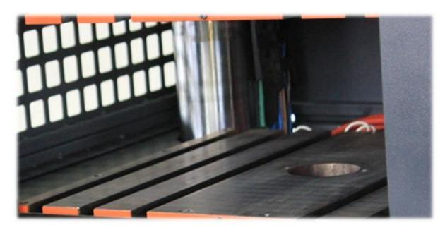
The hydraulically operated center ejector allows you to automatically eject products from the mold. This significantly reduces production time and increases production volume.
