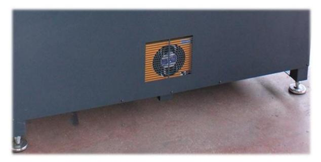
With the oil cooling unit in our presses, the machine automatically cools the hydraulic oil when the temperature exceeds the one you specify, and thus you will not experience any power loss and your felt life will be extended.
