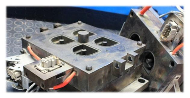
Our presses can optionally be heated directly by attaching a resistance to the mold. The press automatically monitors the resistance and mold temperature, ensuring you get the best product possible.
