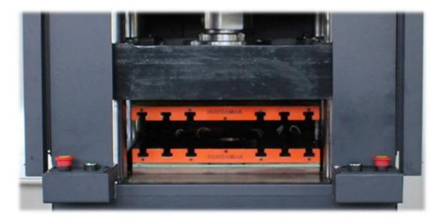
You can adjust all degassing parameters in detail on our presses. Degassing frequency, rise distance, hold at top, and re-press parameters are all customizable.
